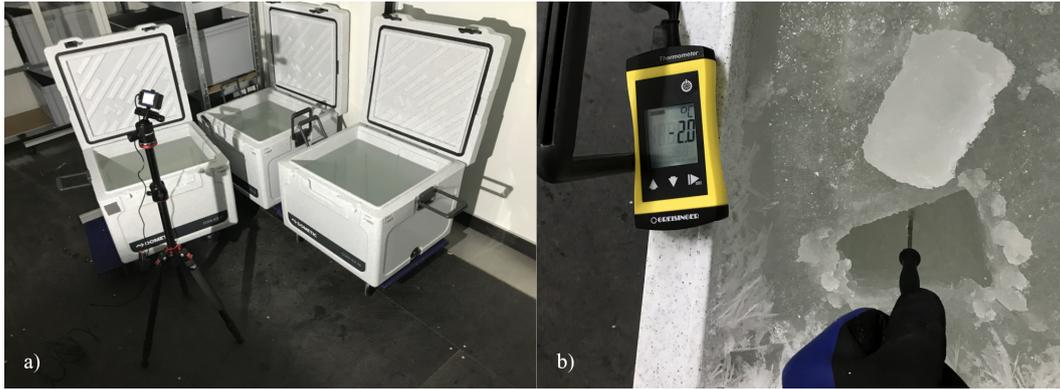
**Figure 6.** a) Experimental setup including the camera to record initial ice formation. b) Example of an ice sample and water temperature measurements.
