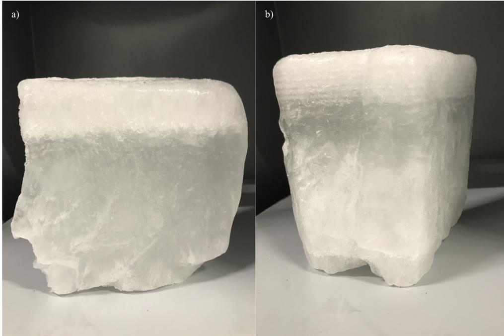
**Figure 7.** Ice samples during different experiments after multiple days of draining. a) Ice after instant flooding. b) Ice after incremental flooding showing multiple thin layers.
